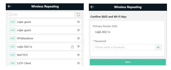
(2) Set the SSID and password and save the settings. Then, the Wi-Fi network will be restarted.
