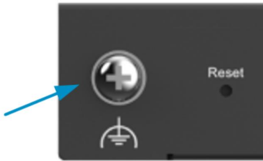
Figure 2-2 Grounding of the Switch
